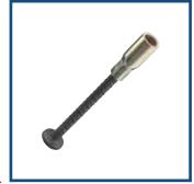
The PFEIFER Allround Anchor long is intended for use as a lifting anchor for front-sided installation in wall-type concrete elements. Through the upset head in combination with the short anchor lengths this anchor – in comparison with other anchor variants – is particularly easy to place in the formwork, even with a dense reinforcement layout.
