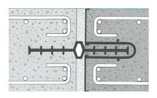
Disposable steel formwork, combined with holder for waterproofing and expansion joint
