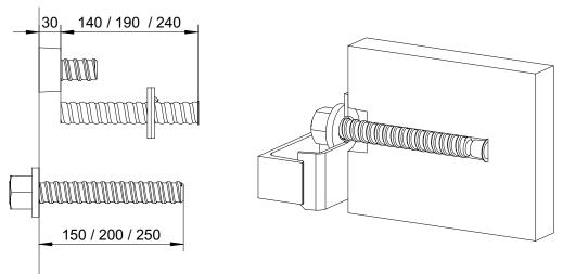
Installation-kit with recoverable clamping flange 30 mm, with bolt with suspension cone Ø 26.5 mm Sleeve length = bolt length -10 mm
