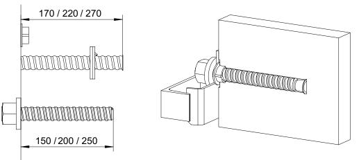
Installation-kit with recoverable clamping flange 30 mm, with hexagonal bolt SW46, Ø 26.5 mm Sleeve length = bolt length –10 mm
