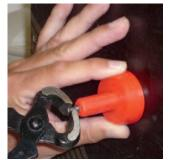
An easy removing oft the nailing flange by the double headed nail
