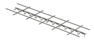
Linear plastic spacer of the lower reinforcement layer. SLALOM is stable, resistant to shifts and fluctuations and can absorb high reinforcement loads. It facilitates its concrete encasement, and prevents void formation or the formation of cracks in the concrete.
