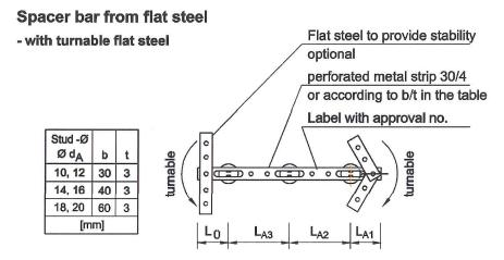
Material: A4 = 1.4571/ 1.4401/ 1.4404 (acc. to EN 10088-5:2009) S 235 JR = 1.0038 (acc.to EN10025-2:2004) DD11 = 1.0332 (acc. to EN10111:2008)
